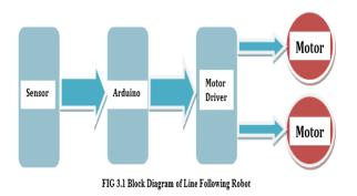
These robots have the capability to detect a black or dark line on a lighter surface depending on the contrast. They estimate whether the line underneath them is shifting toward their left or right as they move over them. Based on that estimation, they give respective signals to the motors to turn left or right so as to maintain a steady center with respect to the line.
